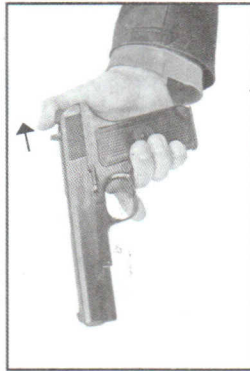
Fig. 4> Blocking the trigger with the hammer lowered
