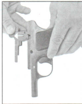
Fig. 9> Separating the trigger mechanism from the frame
