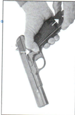
Fig. 5> Taking out the magazine
