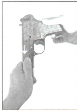
Fig. 8> Separating the slide
